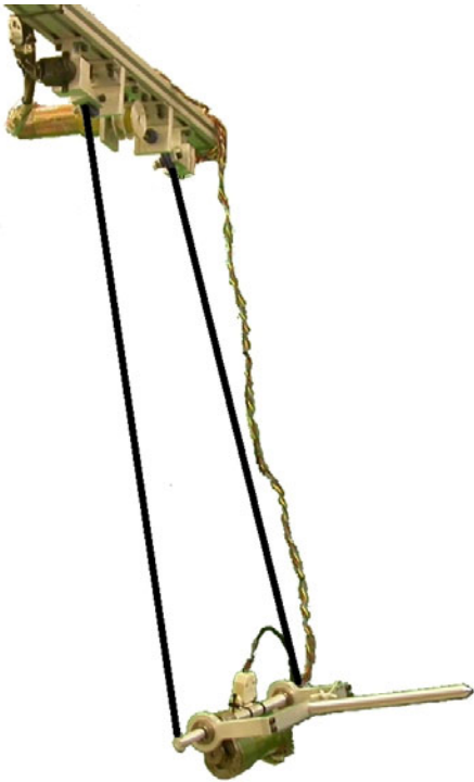
Fig. 4. Prototype of the underactuated cable-driven robot
